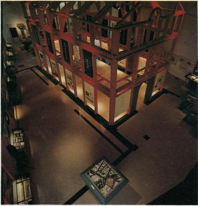
Fixing lighting fittings to a custom-built, free standing structure resolves the perennial problem of how and where to fix and supply energy to the luminaire. From the Prince of Wales "Vision of Britain" Exhibition at the V & A. Lighting designed by Equation Lighting.
